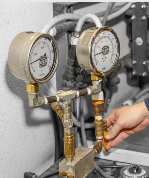
Valves are tested to 1000 PSI and beyond.
