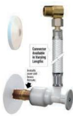
1/2" Nom. Supply Stop with Factory Attached PVC or Braided Flexible Connector x 3/8" Comp. Nut x 1/2" M.I.P. Brass Elbow with Escutcheon. Available with Factory Installed Shut-Off Clip Upon Request for an Additional Cost.
