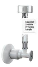
1/2" nom. Supply Stop with Factory Attached PVC or Braided Flexible Connector x 7/8" Reinforced Polymer Ballcock Nut with Escutcheon. Available with Factory Installed Shut-Off Clip Upon Request for an Additional Cost.
