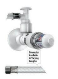
1/2" nom. Supply Stop with Factory Attached PVC or Braided Flexible Connector with Manifold Tee and Hybrid Stainless/Polymer Arrester 3/8" Comp. Nut with Escutcheon.
