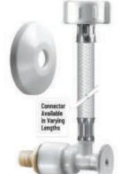
1/2" nom. Expansion Supply Stop with Factory Attached PVC or Braided Flexible Connector x 7/8" Reinforced Polymer Ballcock Nut with Escutcheon. Available with Factory Installed Shut-Off Clip Upon Request for an Additional Cost.
