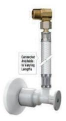
1/2" nom. Supply Stop with Factory Attached PVC or Braided Flexible Connector x 3/8" Comp. Nut x 1/2" M.I.P. Brass Elbow with Escutcheon. Available with factory installed shut-off clip upon request for an additional cost.
