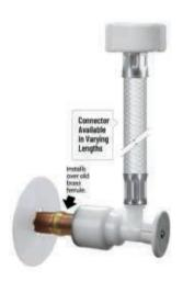
1/2" Nom. Supply Stop with Factory Attached PVC or Braided Flexible Connector x 1/2" Reinforced Polymer IPS Nut with Escutcheon. Sold in Pairs. Upon Request 1/2" Metal IPS Nut may be Substituted for an Additional Cost. Available with Factory Installed Shut-Off Clip Upon Request for an Additional Cost.
