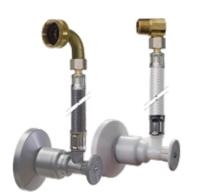
DISHWASHER KIT 1/2" nom. supply stop with factory attached braided or PVC High Performance flexible connector x 3/8" comp. x 3/8" M.I.P. brass elbow or 3/4" Whirlpool elbow with escutcheon.
